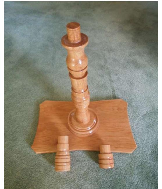
White Oak lumber that sat around for a long time drying in the Michigan air. Each piece was planed and edge joined. Glued sections were fitted with biscuit joiners to add strength.
